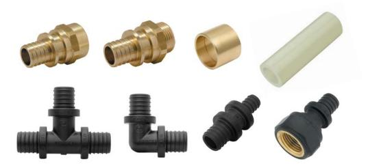
Tight connections without O-rings in the KAN-therm Push System are obtained by means of sliding the brass ring onto the fitting and pipe. The connections do not require any additional sealing, such as Teflon tape or tow. Manifolds and installation cabinets are a supplementation to the system.
