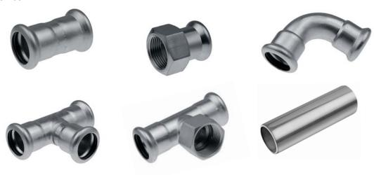
The "press" technology applied in the KAN-therm lnox System provides a quick and reliable performance of connections by means of pressing of fittings with the use of commonly available crimping tools, eliminating the process of threading or welding of the particular elements.
