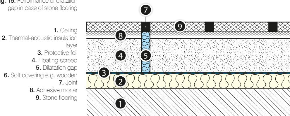
In case of ceramic and stone boards, the distribution of heating plates should already be adjust-
