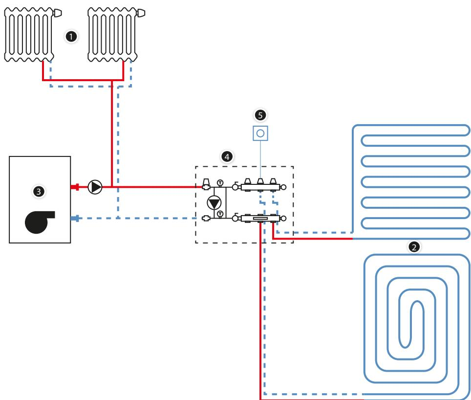
**Fig. 60.** Manifold provided with 77A (or 73A) mixing system
