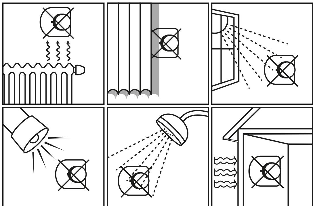
Thermostats mounting should be performed in accordance with the manuals, attached to the product.
