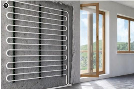
2. Basic elements of wall heating/cooling
