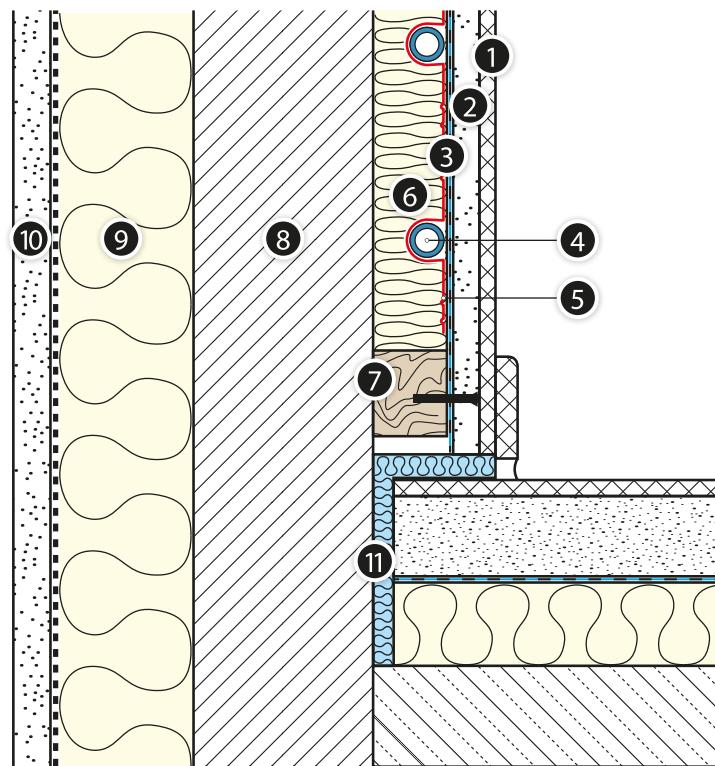
Heating pipes of 12 mm diameter are placed in the channels of KAN-therm TBS 14 boards, equipped with radiators made of steel sheet. TBS 14 boards are mounted between the horizontal strips or 25 × 50 mm steel profiles, to the wall surface. On such a construction a PE foil, which serves as acoustic and damp-proof insulation, is applied, and then plasterboards are mounted to strips.
