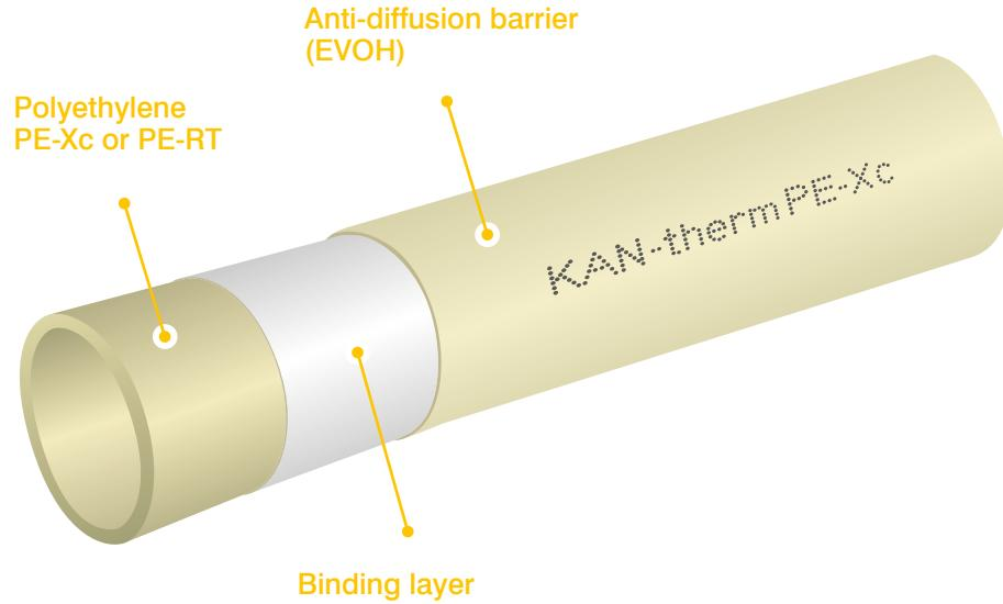
**Fig. 48.** Design of KAN-therm multilayer pipes
