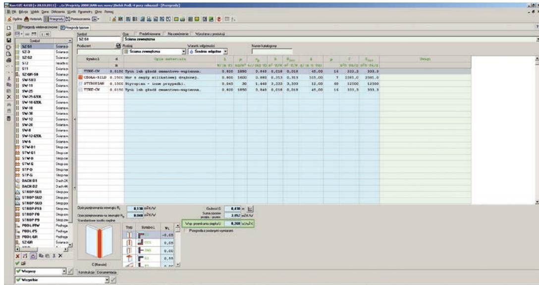
A software package that supports calculations of thermal power demand as well as seasonal heat demand for heating of buildings. Works with the KAN C.O. Graf package.
