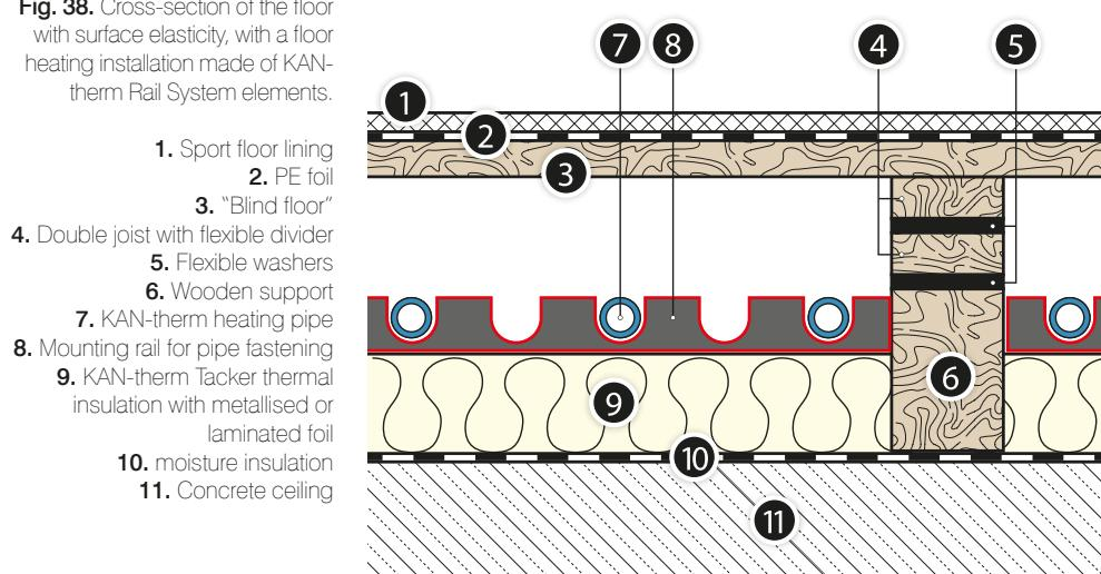
After the arrangement of thermal insulation, holes should be made in it, which shall be used for the accommodation of floor supports in accordance with the recommendations of sports floor supplier. The number of holes and spacing between them depends on the adopted type of a floor.
