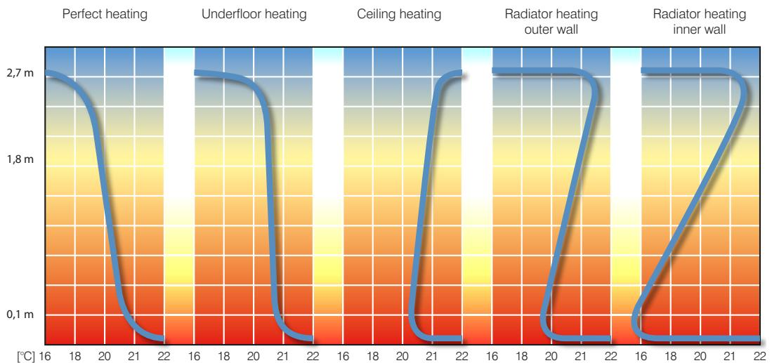
Considerably important, in terms of surface heating comfort, is greatly reduced (compared with radiator heating systems) air convection that causes floating of allergenic dust. Furthermore, surface heating reduces growth of harmful mites due to the low relative humidity at the floor level.
