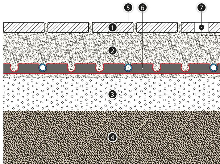
**Fig. 40.** External traffic routes heating (KAN-therm NET System)
