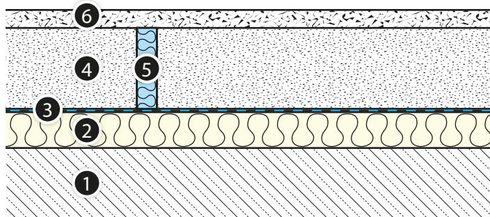
**Fig. 15.** Performance of dilatation gap in case of stone flooring
