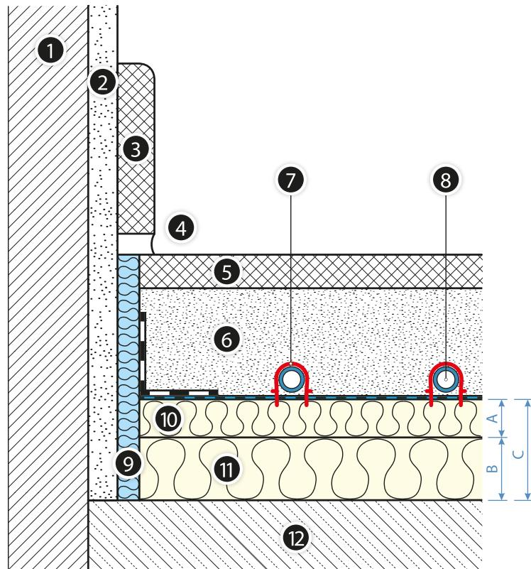
**Fig. 23.** Floor heater with KAN-therm Tacker System board and supplementary insulation and damp-proof coating on the ceiling laid out on the ground
