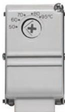
The thermostat is used as a protection against exceeding of the preset temperature in the radiator or floor heating installations. The device is mounted directly on the supplying or return pipe - depending on the needs. In case of reaching temperature value set on the thermostat, the device automatically turns off the circulating pump. Temperature presetting range 50 – 95°C.
