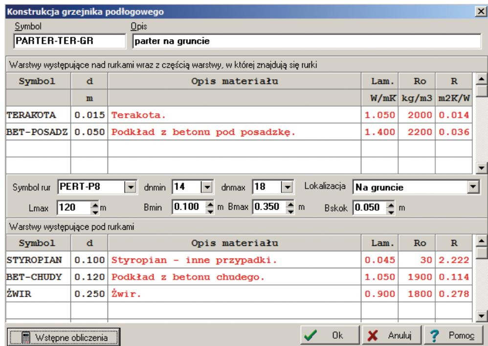
Once the floor heater design is entered, initial calculation of the heater output can be calculated forthwith (Fig. 78). This will enable an approximate determination of heater thermal efficiency, floor surface temperature and other parameters. The results may prove very helpful for designing heaters in specific premises.
