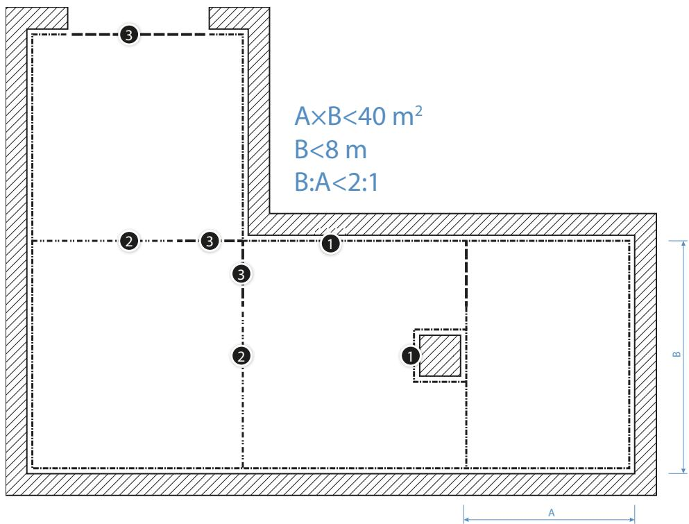
**Fig. 18.** Correct and incorrect distribution of heating field with a dilatation gap
