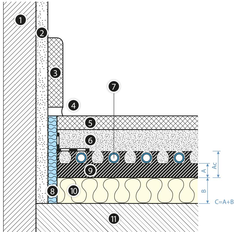
**Fig. 27.** Floor heater with KAN-therm Profil3 System board and supplementary insulation on the ceiling above the internal not heated room and on the ceiling laid out on the ground (damp insulation required!)
