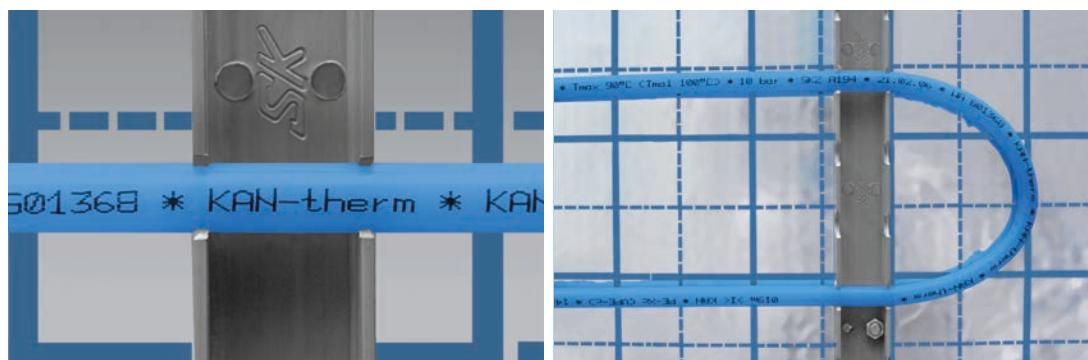
Heating pipes of 12 or 14 mm diameter are mounted on the wall in mounting strip, and then they are covered with a plaster layer of a total thickness of approx. 30-35 mm, forming a hotplate. The minimum plaster layer thickness over the pipe surface is 10 mm.
