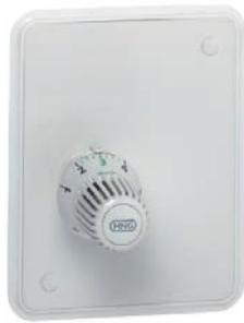
The device controlling temperature in a room regulates the flow of medium through single floor heating circuit, without additional heaters, depending on ambient temperature. Room set can be mounted both on the supply and return in floor heating circuit. Thermostat receives the ambient temperature and properly regulates the flow of water in a heating circuit.
