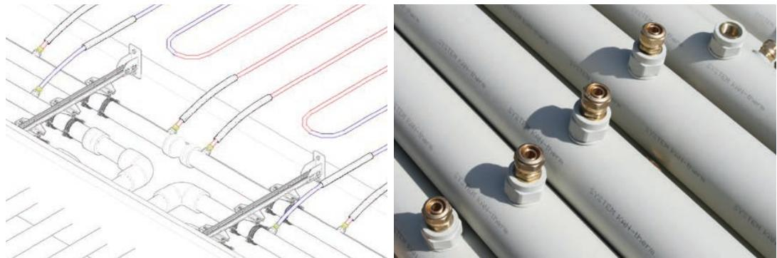
Possible configuration of KAN-therm PE-RT 18 x 2 mm heating pipes connection to KAN-therm PP Glass collector made of pipes of diameter 50 mm:
