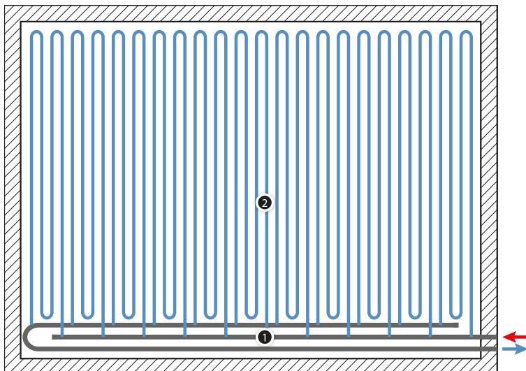
In the Tichelmann system, which guarantees even pressure distribution in the installation, heating circuits are connected through a three-way adapter (or KAN-therm PP saddle joints) to the supplying and return connectors laid under the floor, along the shorter and longer sides of sports hall.
