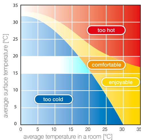
Surface heating/cooling systems are low temperature systems. Average temperature of heating/cooling surface is only slightly higher (or lower for cooling) than the air temperature within the space. For surface heating, temperature of 20°C provides the same thermal comfort as 21- 22°C achieved with traditional radiators on convection heaters.
