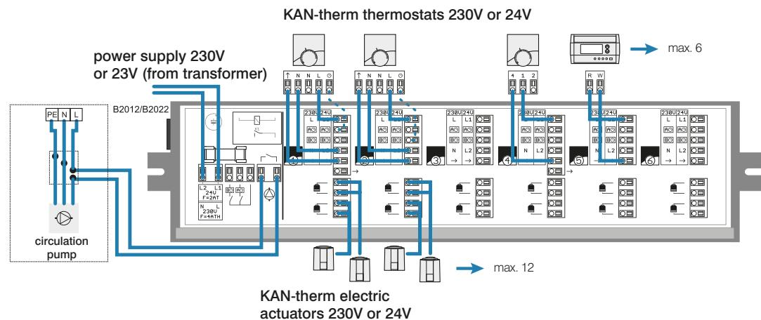
Normally one thermostat can control one or two actuators. If a jumper (A) is used, one thermostat can control 3 or 4 actuators.
