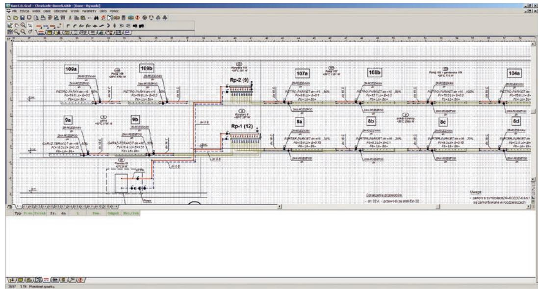
KAN C.O. Graf enables projecting the results of calculations onto floor plans (**Fig. 81**). To do this, draw a floor plan and then project heaters, pipes and other system components onto the plan. For simple shapes the software will draw underfloor heating coils. Once the calculations are complete, the software will describe the size of the heater and draw them to scale, it will provide pipe diameters and valve settings.
