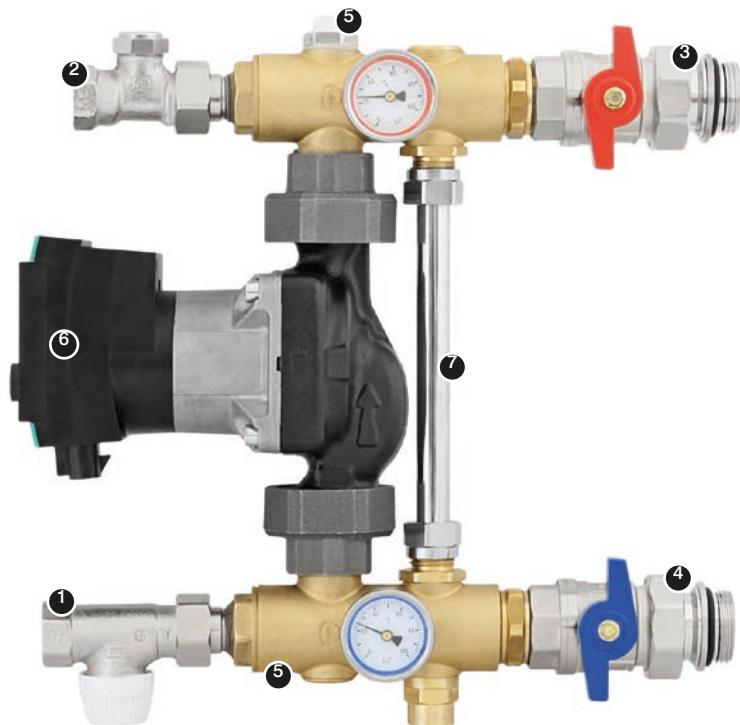
Mixing system is composed of a pump (three-stage or stepless depending on a version), ZR control valve, regulated by-pass, ZT thermostatic valve, 1" terminals to manifold and high-temperature installation, as well as 2 thermostats.
